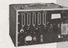
Portable Pulse Analyzer—transistorized, battery operated unit displaying pulse rate, width, and rise times.
