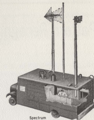
Spectrum Surveillance System—mobile RFI monitoring facility for missile test range, 0.5 mc to 10.7 Gc, includes beacon checkout tester.
