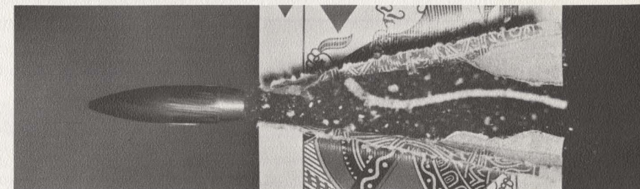
A 30 caliber bullet cuts easily across this playing card. This picture was taken at MIT by Dr. Edgerton using an EG&G Microflash. In a darkened room the pre-aimed rifle is fired. Its sound, picked up by a microphone, triggers the ultra-bright, short-duration flashtube in the Microflash. The camera shutter is open during the entire sequence.
