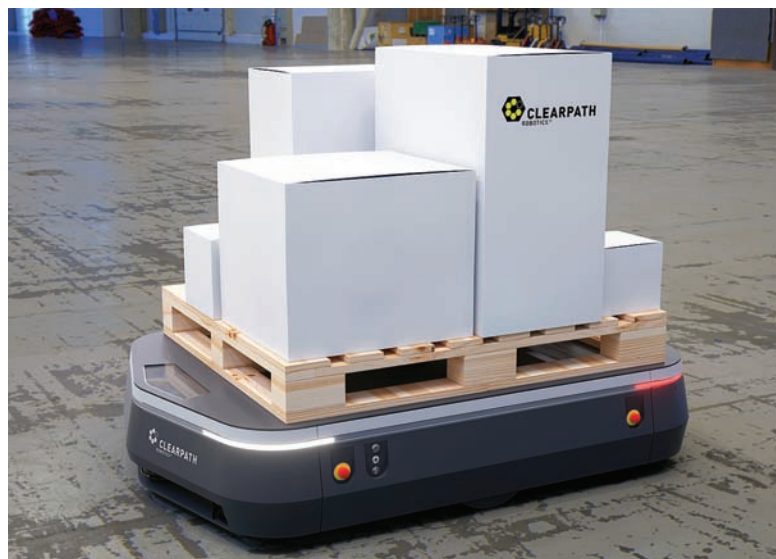
Clearpath's Otto 1500 self-driving transporter (above) is designed to move materials around a warehouse, avoiding obstacles while taking the fastest possible route to its destination. IEEE Member Ryan Gariepy (below) cofounded Clearpath while pursuing a bachelor's degree.
