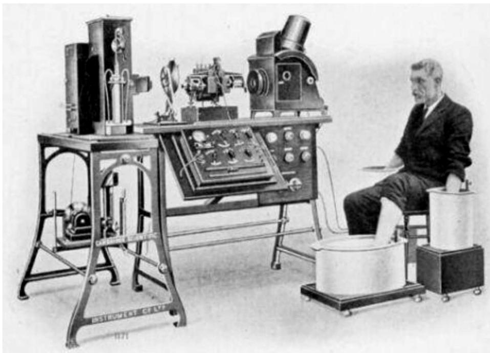
**Fig. 5.** Complete instrumentation for ECG. Courtesy of the University of Leiden, The Netherlands.
