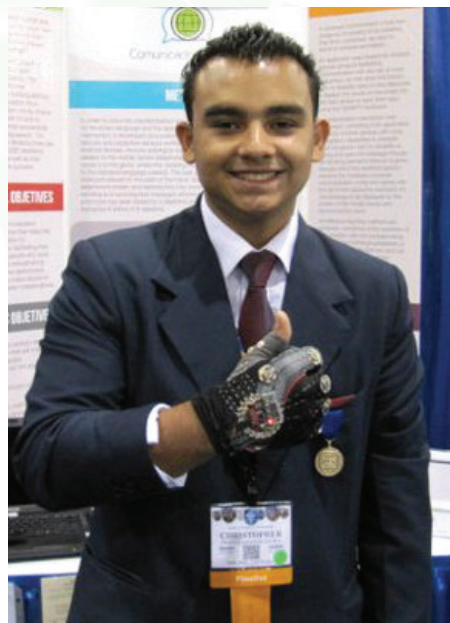
IEEE Presidents' Scholarship winner, Portocarrero-Mora, created a communication device that transmits voice or text from a cellphone or tablet computer to a glove embedded with vibrating sensors that the deaf and blind can interpret.
