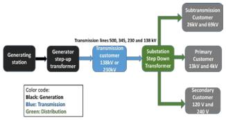
Figure 1 Basic electric system structure [11]
