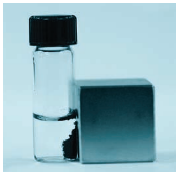
Jin-Woo Kim's system uses a magnet and clusters of multiwalled carbon nanotubes. The clusters capture bacteria such as E. coli , and as illustrated above, the rare earth element neodymium magnet attracts the nanotubes.
