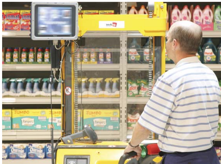
Relying on a scanner that reads the RFID label on each product, a store manager at a Metro "future store" will be able to tell quickly what's on his shelves and what's been sold.
