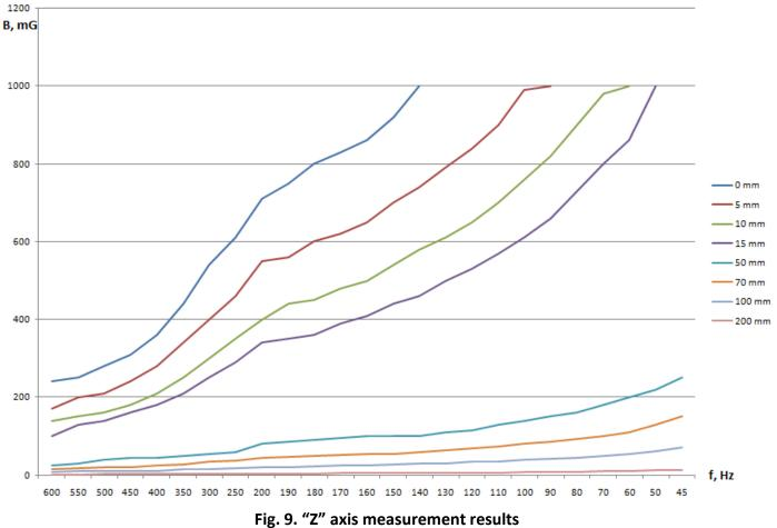
According to Table 2, the measurement results did not exceed the exposure limits (1 G = 0.0001 T).
