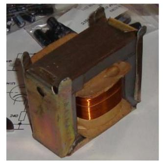
Fig. 4. Output audio transformer
