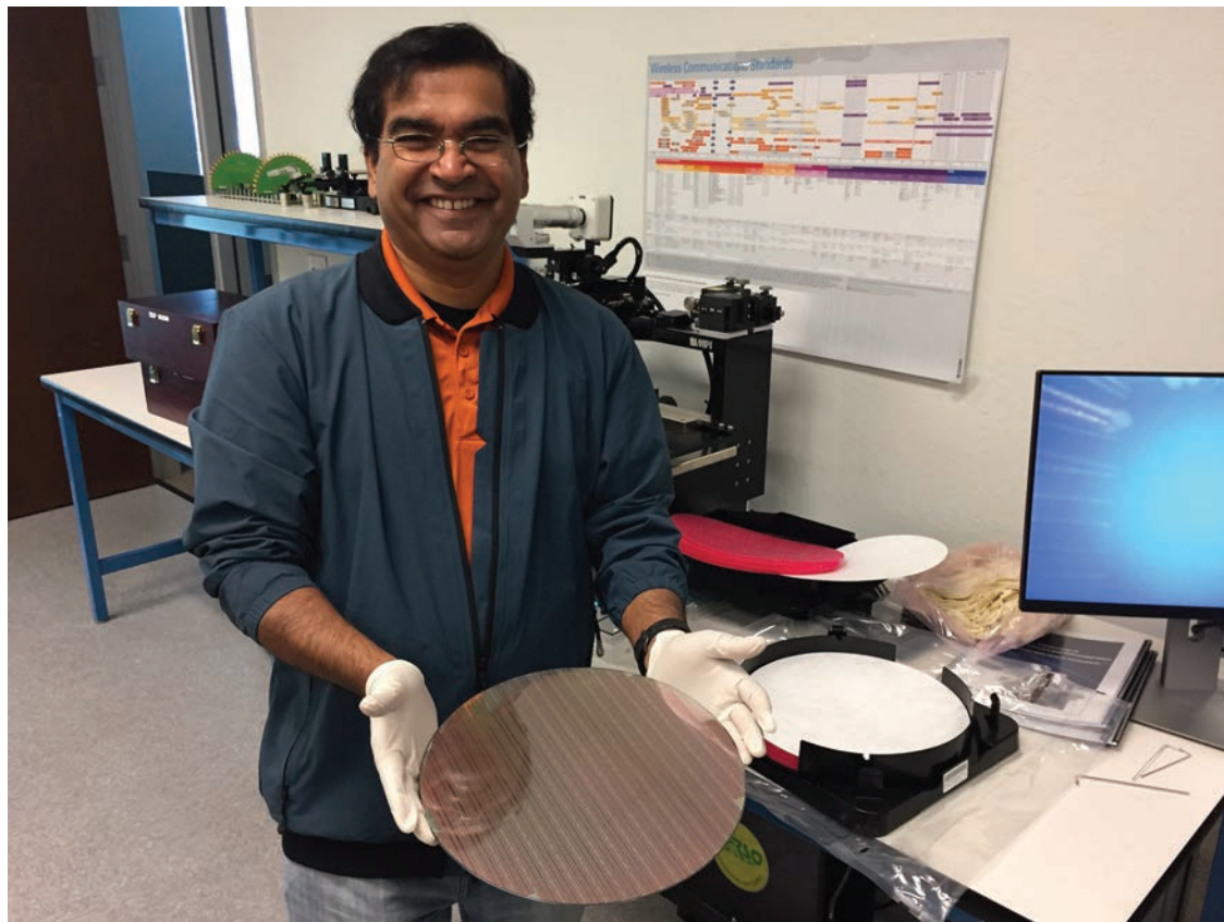
IEEE Fellow Joy Laskar holds a CMOS wafer containing Maja Systems' 60-gigahertz transceiver chips. The wafer yields several thousand chips, each with a modulation engine, and is made in a standard digital process modified for millimeter wave frequencies.
