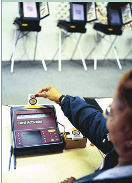
A voter inserts her voter-identification card into a management terminal that will clear her to use one of the touch-screen voting machines in the background.
