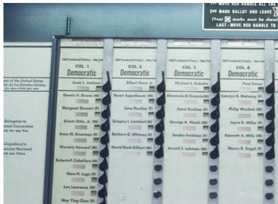
The IEEE 1583 e-voting standard will specify performance guidelines for electronic machines that will replace mechanical machines such as this lever-actuated device still in use in New York City.
