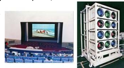
400-inch screen and twelve CRT projectors 1985.
