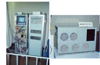
MUSE (Multiple Sub-Nyquist Sampling Encoding), a bandwidth compression system, 1983.
