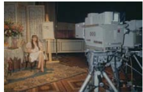
HDTV camera composed of 1-inch DIS (Diode-gun Impregnated-cathode SATICON) tube, at a CBS studio, 1982.
