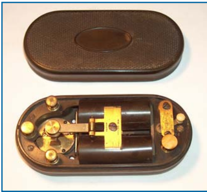
An early wiretapping technology: the Telegraph Lineman’s Test Set. Photo courtesy of John Casale www.telegraph-history.org
