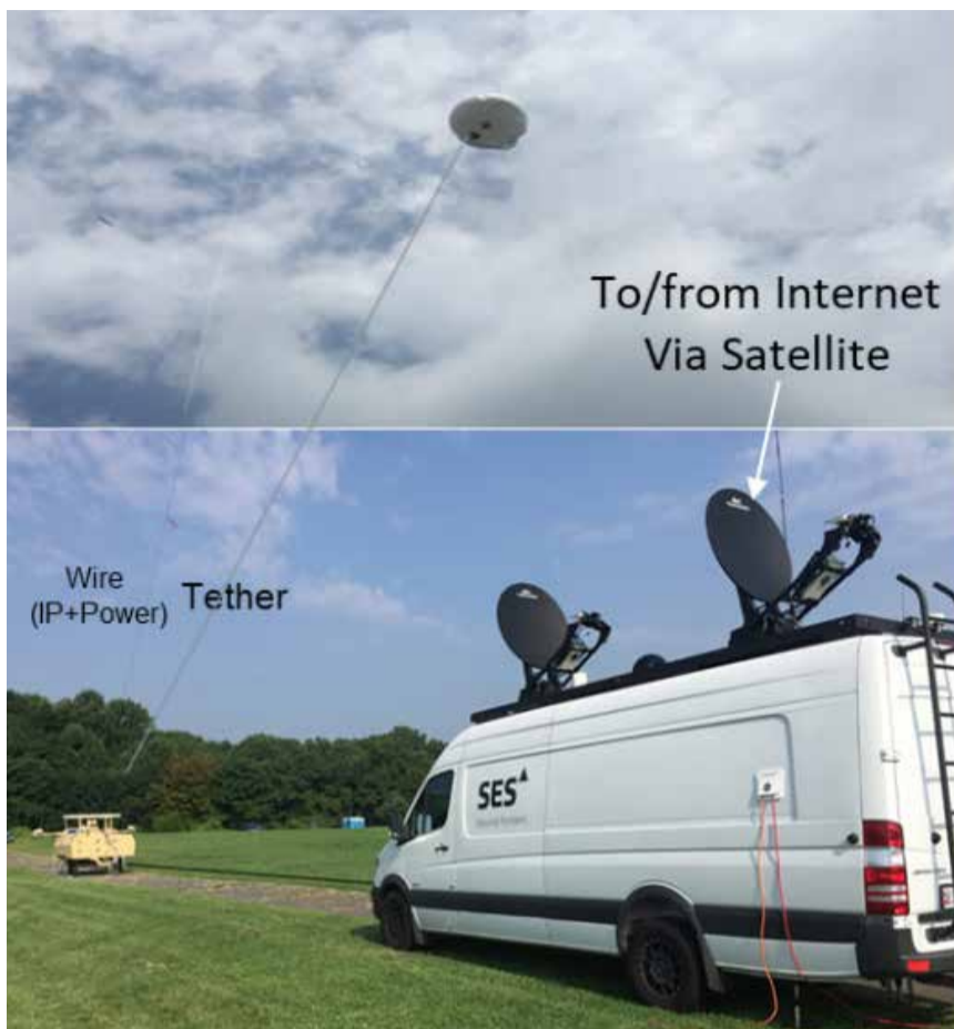
Fig. 4: A aerial node connected to the terrestrial broadband network through a tethered backhaul and satellite service. (Image Courtesy: Mutualink Inc.)
