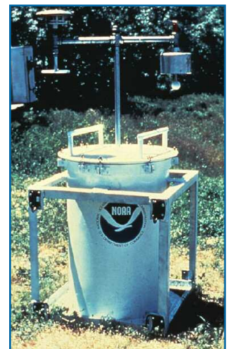
TOTO – Torable Tornado Observatory – an instrument package designed to be placed in the path of tornadoes. Photo courtesy of National Oceanographic and Atmospheric Administration
