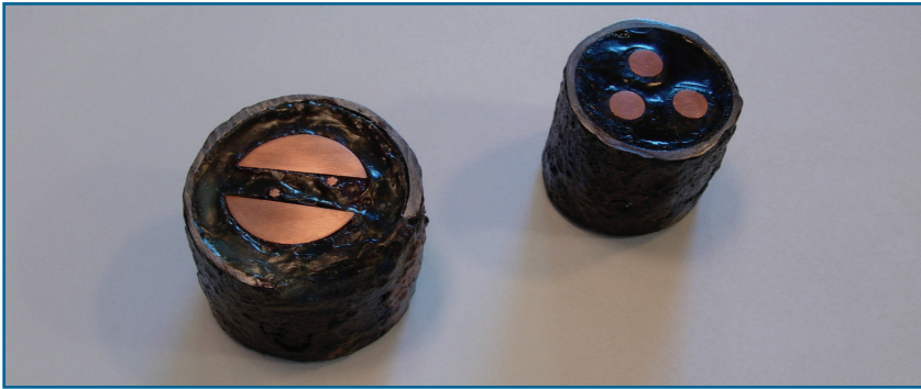
Sections of two-conductor and three-conductor transmission cables from Edison's Pearl Street Generating Station. These cables were dug up recently from under the streets of lower Manhattan.
