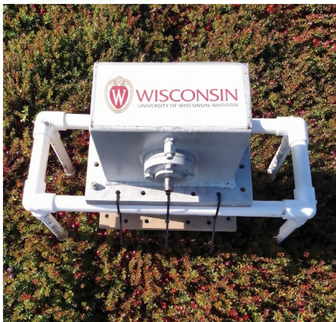
To help Ocean Spray farmers count cranberries, researchers at the University of Wisconsin in Madison developed a prototype for a microwave sensing system that can scan a small part of a cranberry bog at a time. The system then estimates the number of berries—a task that now requires manual labor.
