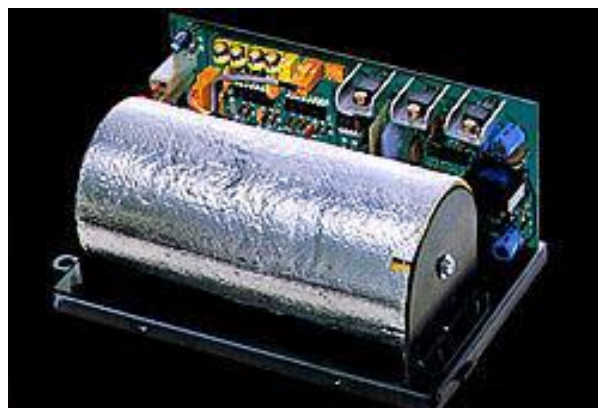
Fig. 10: Outside construction of gas-rate gyro sensor
