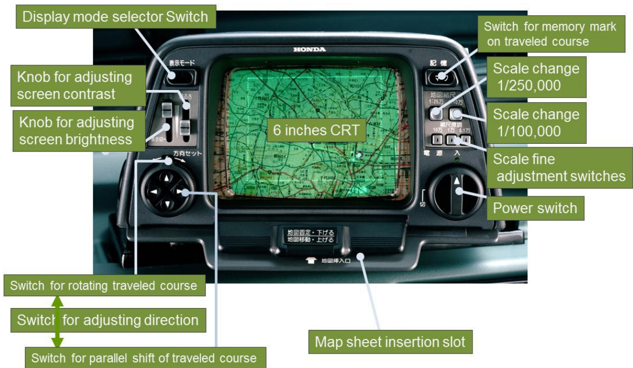
Fig. 5: Switches configuration of display equipment (front view)
