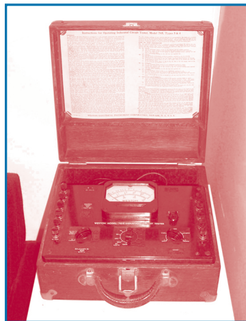
Weston Model 785 Industrial Circuit tester, donated to the IEEE Archives by IEEE life member Raymond Stahl.
