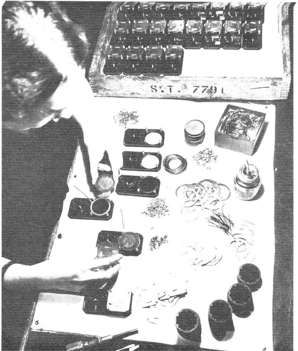
An Exposure Meter's Nervous System . . . is here being assembled. In her hand this girl holds the meter's round flat electric eye which, when properly sandwiched and clamped between lens, grid, electrode, gasket, and terminals, will become a Weston Photronic Cell, capable of translating the light that strikes it into current which it will shoot through its wire tail into the Weston movement later to stand beside it on the oblong bakelite base. And camera fans, watching the movement's pointer, will know how wide their lenses should be opened and how fast their shutters should be clicked.
