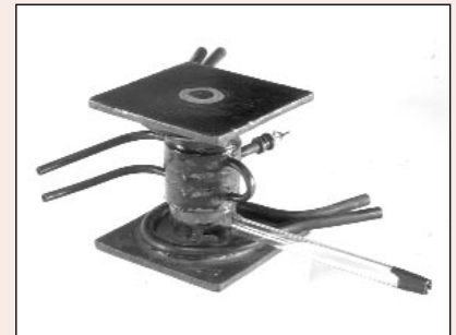
The original 1940 cavity magnetron developed by J.T. Randall and Henry Boot. It was crucial to the success of the Allies' radar program and makes the microwave oven possible. Courtesy: Science Museum/Science & Society Picture Library.
