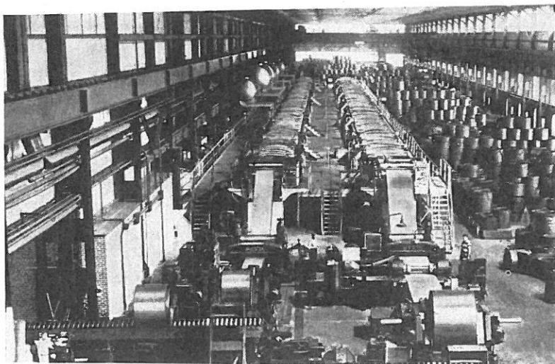
Two new continuous pickling lines process strip from the 68 in. mill before the material passes on to the cold reduction mill.
