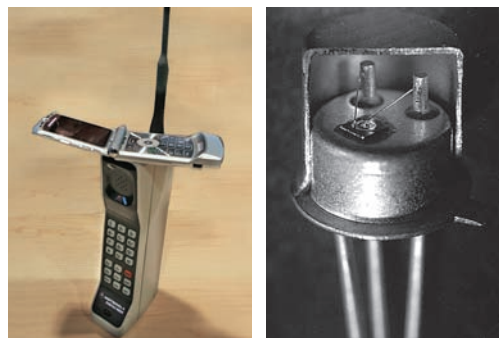
Clockwise from top: Geographic map of the ARPANET; Fairchild Semiconductor's first commercial planar transistor; Motorola's Razr cellphone on top of the company's first cellphone, a DynaTAC 8000X.
