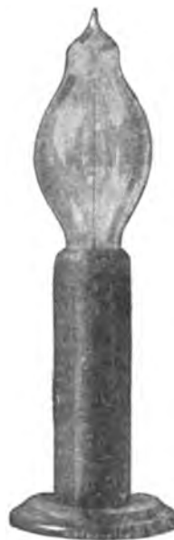
FIG. 26A. LAMP WITH ONE FILAMENT, ONE INSIDE AND ONE OUTSIDE CONDENSER COATING.
