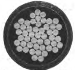
Feeder Cable, Brooklyn Edison Electric Light Co.
