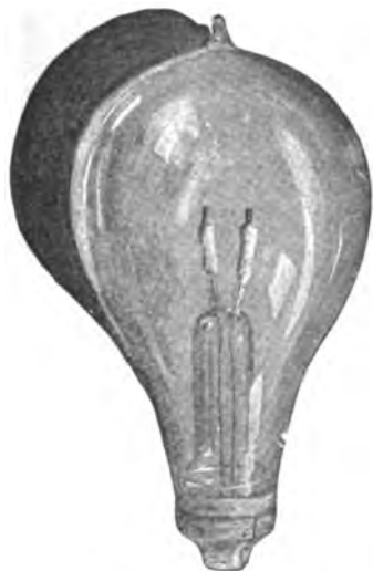
FIG. 22.—LAMP WITH TWO REFRACTORRY BLOCKS IN HIGHEST VACUUM.
