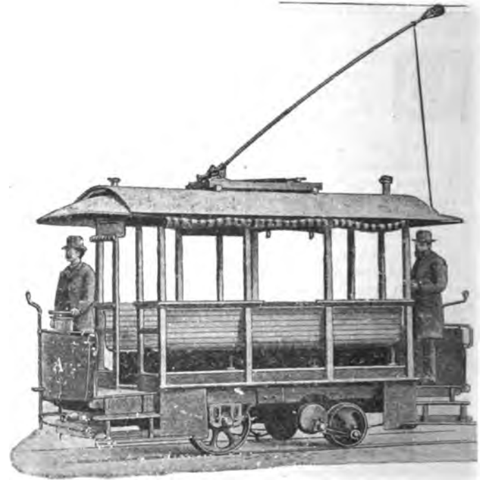
FIG. 4.—EICKEMEYER-FIELD DIRECT CONNECTED MOTOR.
