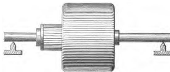
FIG. 9.—METHOD OF BALANCING ARMATURE.
