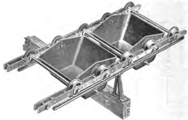
FIG. 2.—DETAILS OF HUNT COAL CONVEYER.
