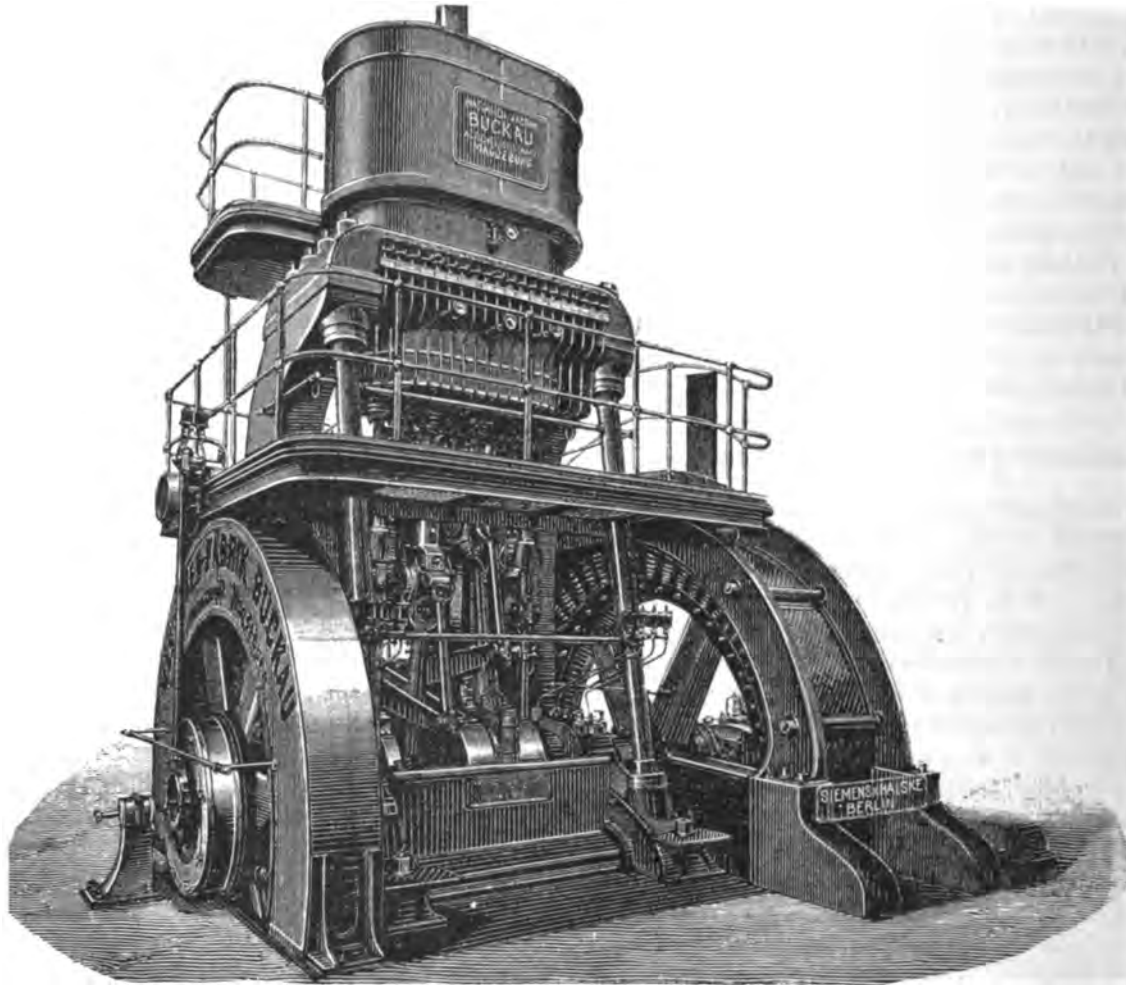
FIG. 1.—SIEMENS & HALSKE ALTERNATOR DRIVEN BY TRIPLE EXPANSION CONDENSING ENGINE.
