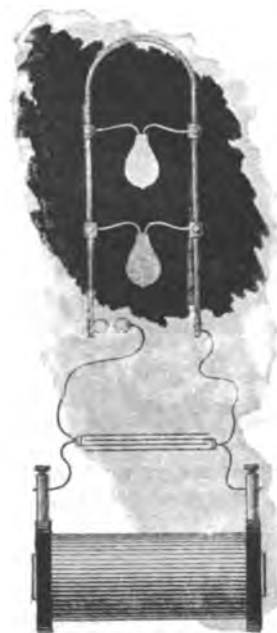
FIG. 33.—LAMP KEPT AT INCANDESCENCE ACROSS A THICK COPPER BAR—SHOWING NODES.
