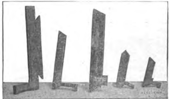
FIG. 3.—VARIOUS FORMS OF COMMUTATOR SEGMENTS.
