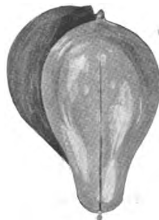
FIG. 23.—LAMP WITH SINGLE STRAIGHT FILAMENT AND ONE LEADING-IN WIRE.
